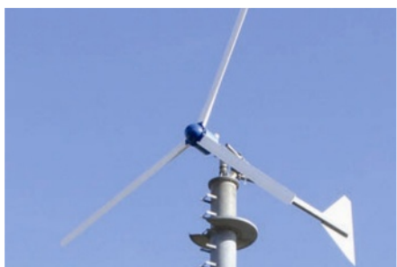
Alize on a free standing pole with additional steps. This turbine electrifies a consultancy office.
