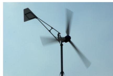
Montana on a guyed pole. This turbine is used for home electrification in The Netherlands.
